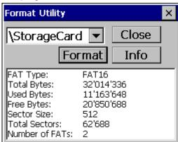
The Flash card drive can be selected in the top left selection field. The lower display field shows the information about the selected drive. This information includes details such as FAT type, total memory, currently used memory etc. Much of the information is not normally required.
